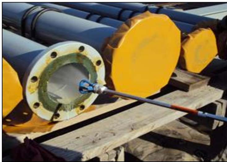
Figure4: Pipeline Preservation using Liquid VCI
